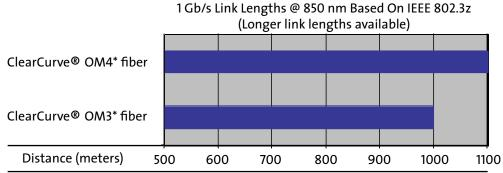
Link lengths as characterized in IEEE 802.3z (Gigabit Ethernet) and IEEE 802.3ae (10 Gigabit Ethernet) for ClearCurve multimode fiber-specific bandwidth metrics and standards compliant components. 1 Gb/s and 10 Gb/s link lengths shown for ClearCurve OM4 fiber and 1 Gb/s shown for ClearCurve OM3 fiber systems require cable attenuation ≤ 3.0 dB/km and total connector loss ≤ 1.0 dB.
