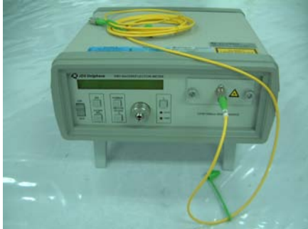
Fig.2-3 JDSU RM-3 Backreflection Meter
