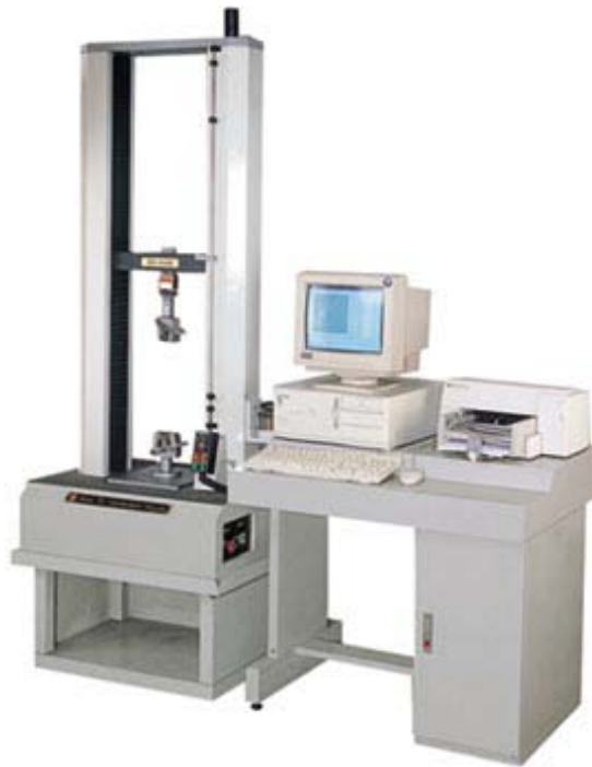
Fig.2-1 Computer control materials testing system
