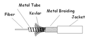
Fig.1 The schematic diagram of duplex armored optical fiber cable
